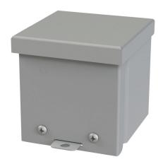
Saginaw enclosure, NEMA 3R, 4 x 4 x 4in (HxWxD), wall mount, carbon steel, ANSI 61 gray, powder coat finish, screw cover, padlock hasp and staple.
