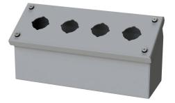
Saginaw pushbutton consolet, 4 holes, 30mm, NEMA 4/12/13, 4 x 10 x 5in (HxWxD), wall mount, carbon steel, ANSI 61 gray, powder coat finish, screw cover.
