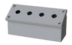
Saginaw pushbutton consolet, 4 holes, 22mm, NEMA 4/12/13, 4 x  $10 \times 5$ in (HxWxD), wall mount, carbon steel, ANSI 61 gray, powder coat finish, screw cover.
