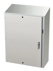
Saginaw Enviroline series disconnect enclosure, slope top, NEMA 3R/4/4X/12/13, right flange, 48 x 37 x 16in (HxWxD), wall mount, 304 stainless steel, #4 brush finish, single-door, 3-point padlocking handle, purchase subpanel separately.
