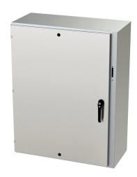
Saginaw Enviroline series disconnect enclosure, NEMA 3R/4/4X/12/13, right flange, 48 x 37 x 16in (HxWxD), wall mount, 304 stainless steel, #4 brush finish, single-door, 3-point padlocking handle, purchase subpanel separately.
