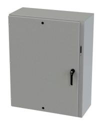
Saginaw Enviroline series disconnect enclosure, NEMA 3R/4/12/13, right flange, 48 x 37 x 16in (HxWxD), wall mount, carbon steel, ANSI 61 gray, powder coat finish, single-door, 3-point padlocking handle, purchase subpanel separately.
