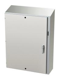
Saginaw Enviroline series disconnect enclosure, slope top, NEMA 3R/4/4X/12/13, right flange, 48 x 37 x 12in (HxWxD), wall mount, 304 stainless steel, #4 brush finish, single-door, 3-point padlocking handle, purchase subpanel separately.
