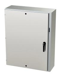
Saginaw Enviroline series disconnect enclosure, NEMA 3R/4/4X/12/13, right flange, 48 x 37 x 12in (HxWxD), wall mount, 304 stainless steel, #4 brush finish, single-door, 3-point padlocking handle, purchase subpanel separately.
