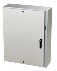
Saginaw Enviroline series disconnect enclosure, NEMA 3R/4/4X/12/13, right flange, 48 x 37 x 12in (HxWxD), wall mount, 316L stainless steel, #4 brush finish, single-door, 3-point padlocking handle, purchase subpanel separately.
