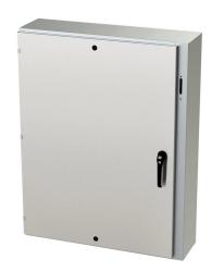
Saginaw Enviroline series disconnect enclosure, NEMA 3R/4/4X/12/13, right flange, 48 x 37 x 10in (HxWxD), wall mount, 316L stainless steel, #4 brush finish, single-door, 3-point padlocking handle, purchase subpanel separately.
