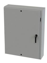
Saginaw Enviroline series disconnect enclosure, NEMA 3R/4/12/13, right flange, 48 x 37 x 10in (HxWxD), wall mount, carbon steel, ANSI 61 gray, powder coat finish, single-door, 3-point padlocking handle, purchase subpanel separately.
