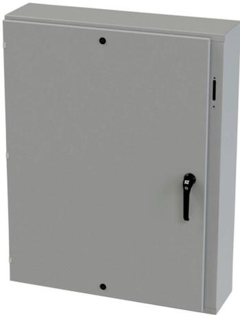
Saginaw Enviroline series disconnect enclosure, NEMA 3R/4/12/13, right flange, 48 x 37 x 10in (HxWxD), wall mount, carbon steel, ANSI 61 gray, powder coat finish, single-door, 3-point padlocking handle, purchase subpanel separately.
