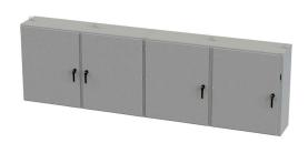
Saginaw disconnect enclosure, NEMA 3R/12/13, right flange, 48 x 158 x 18in (HxWxD), freestanding/wall-mount, carbon steel, ANSI 61 gray, powder coat finish, 4-door, 3-point padlocking handle, purchase subpanel separately.
