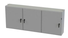
Saginaw disconnect enclosure, NEMA 3R/12/13, right flange, 48 x 118 x 18in (HxWxD), freestanding/wall-mount, carbon steel, ANSI 61 gray, powder coat finish, 3-door, 3-point padlocking handle, purchase subpanel separately.
