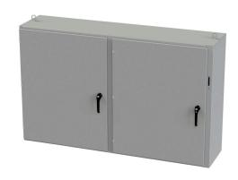
Saginaw disconnect enclosure, NEMA 3R/12/13, right flange, 48 x 78 x 18in (HxWxD), freestanding/wall-mount, carbon steel, ANSI 61 gray, powder coat finish, 2-door, 3-point padlocking handle, purchase subpanel separately.
