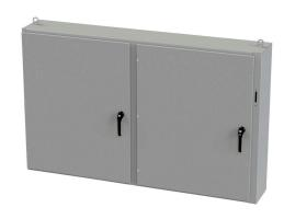
Saginaw disconnect enclosure, NEMA 3R/12/13, right flange, 48 x 78 x 12in (HxWxD), freestanding/wall-mount, carbon steel, ANSI 61 gray, powder coat finish, 2-door, 3-point padlocking handle, purchase subpanel separately.
