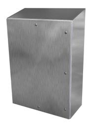
Saginaw sanitary enclosure, slope top, NEMA 3R/4/4X/12,  $48 \times 36 \times 16$  in (HxWxD), wall mount, 304 stainless steel, #4 brush finish, single-door, 1/4-turn sanitary stainless steel latch.
