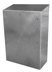
Saginaw sanitary enclosure, slope top, NEMA 3R/4/4X/12, 48 x 36 x 16in (HxWxD), wall mount, 304 stainless steel, #4 brush finish, single-door, 1/4-turn sanitary stainless steel latch.
