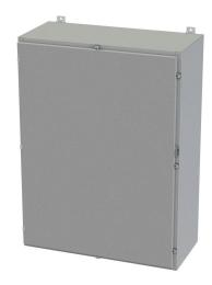
Saginaw enclosure, NEMA 3R/4/12/13, 48 x 36 x 16in (HxWxD), wall mount, carbon steel, ANSI 61 gray, powder coat finish, single-door, plated steel clamps, padlock hasp and staple.
