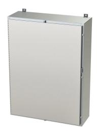
Saginaw enclosure, NEMA 3R/4/4X/12/13, 48 x 36 x 12in (HxWxD), wall mount, 316L stainless steel, #4 brush finish, single-door, stainless steel clamps, padlock hasp and staple.
