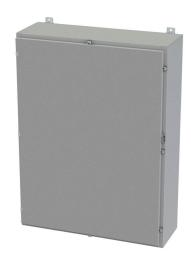
Saginaw enclosure, NEMA 3R/4/12/13, 48 x 36 x 12in (HxWxD), wall mount, carbon steel, ANSI 61 gray, powder coat finish, single-door, plated steel clamps, padlock hasp and staple.
