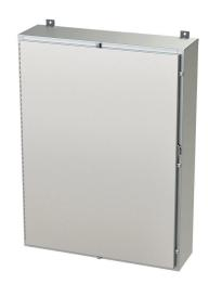
Saginaw enclosure, NEMA 3R/4/4X/12/13, 48 x 36 x 10in (HxWxD), wall mount, 304 stainless steel, #4 brush finish, single-door, stainless steel clamps, padlock hasp and staple.
