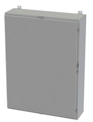
Saginaw enclosure, NEMA 3R/4/12/13, 48 x 36 x 10in (HxWxD), wall mount, carbon steel, ANSI 61 gray, powder coat finish, single-door, plated steel clamps, padlock hasp and staple.
