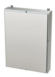
Saginaw enclosure, NEMA 3R/4/4X/12/13, 48 x 36 x 8in (HxWxD), wall mount, 304 stainless steel, #4 brush finish, single-door, stainless steel clamps, padlock hasp and staple.
