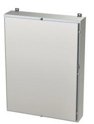
Saginaw enclosure, NEMA 3R/4/4X/12/13, 48 x 36 x 8in (HxWxD), wall mount, 316L stainless steel, #4 brush finish, single-door, stainless steel clamps, padlock hasp and staple.
