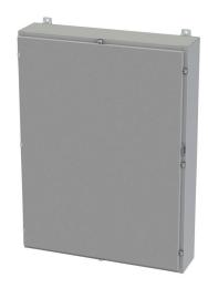
Saginaw enclosure, NEMA 3R/4/12/13, 48 x 36 x 8in (HxWxD), wall mount, carbon steel, ANSI 61 gray, powder coat finish, single-door, plated steel clamps, padlock hasp and staple.
