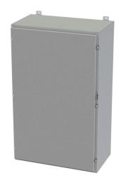
Saginaw enclosure, NEMA 3R/4/12/13, 48 x 30 x 16in (HxWxD), wall mount, carbon steel, ANSI 61 gray, powder coat finish, single-door, plated steel clamps, padlock hasp and staple.
