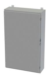
Saginaw enclosure, NEMA 3R/4/12/13, 48 x 30 x 10in (HxWxD), wall mount, carbon steel, ANSI 61 gray, powder coat finish, single-door, plated steel clamps, padlock hasp and staple.
