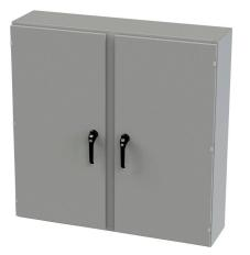
Saginaw Enviroline series enclosure, NEMA 3R/4/12/13, 48 x 48 x 12in (HxWxD), wall mount, carbon steel, ANSI 61 gray, powder coat finish, 2-door, 3-point keylocking/padlocking combo handle.
