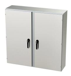
Saginaw Enviroline series enclosure, NEMA 3R/4/4X/12/13, 48 x 48 x 12in (HxWxD), wall mount, 304 stainless steel, #4 brush finish, 2-door, 3-point keylocking/padlocking combo handle.
