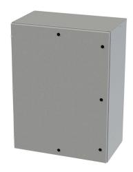
Saginaw Enviroline series enclosure, NEMA 3R/4/12/13, 48 x 36 x 20in (HxWxD), wall mount, carbon steel, ANSI 61 gray, powder coat finish, single-door, 1/4-turn semi-flush latch.
