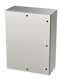
Saginaw Enviroline series enclosure, NEMA 3R/4/4X/12/13, 48 x 36 x 16in (HxWxD), wall mount, 304 stainless steel, #4 brush finish, single-door, 1/4-turn semi-flush latch.
