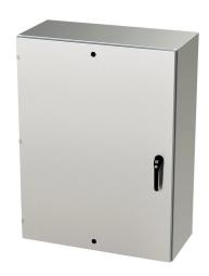
Saginaw Enviroline series enclosure, NEMA 3R/4/4X/12/13, 48 x 36 x 16in (HxWxD), wall mount, 304 stainless steel, #4 brush finish, single-door, 3-point keylocking/padlocking combo handle.
