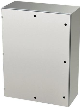
Saginaw Enviroline series enclosure, NEMA 3R/4/4X/12/13, 48 x 36 x 16in (HxWxD), wall mount, 316L stainless steel, #4 brush finish, single-door, 1/4-turn semi-flush latch.
