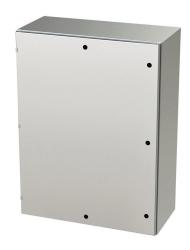
Saginaw Enviroline series enclosure, NEMA 3R/4/4X/12/13, 48 x 36 x 16in (HxWxD), wall mount, 316L stainless steel, #4 brush finish, single-door, 1/4-turn semi-flush latch.
