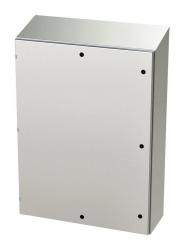
Saginaw Enviroline series enclosure, slope top, NEMA 3R/4/4X/12/13, 48 x 36 x 12in (HxWxD), wall mount, 304 stainless steel, #4 brush finish, single-door, 1/4-turn semi-flush latch.
