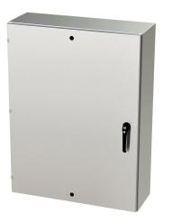
Saginaw Enviroline series enclosure, NEMA 3R/4/4X/12/13, 48 x 36 x 12in (HxWxD), wall mount, 304 stainless steel, #4 brush finish, single-door, 3-point keylocking/padlocking combo handle.
