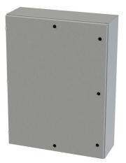
Saginaw Enviroline series enclosure, NEMA 3R/4/12/13, 48 x 36 x 12in (HxWxD), wall mount, carbon steel, ANSI 61 gray, powder coat finish, single-door, 1/4-turn semi-flush latch.
