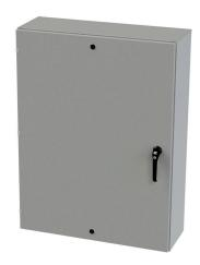
Saginaw Enviroline series enclosure, NEMA 3R/4/12/13, 48 x 36 x 12in (HxWxD), wall mount, carbon steel, ANSI 61 gray, powder coat finish, single-door, 3-point keylocking/padlocking combo handle.
