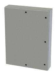
Saginaw Enviroline series enclosure, NEMA 3R/4/12/13,  $48 \times 36 \times 8$  in (HxWxD), wall mount, carbon steel, ANSI 61 gray, powder coat finish, single-door, 1/4-turn semi-flush latch.
