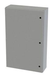
Saginaw Enviroline series enclosure, NEMA 3R/4/12/13, 48 x 30 x 10in (HxWxD), wall mount, carbon steel, ANSI 61 gray, powder coat finish, single-door, 1/4-turn semi-flush latch.
