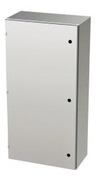
Saginaw Enviroline series enclosure, NEMA 3R/4/4X/12/13, 48 x 24 x 12in (HxWxD), wall mount, 304 stainless steel, #4 brush finish, single-door, 1/4-turn semi-flush latch.
