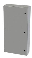
Saginaw Enviroline series enclosure, NEMA 3R/4/12/13, 48 x 24 x 8in (HxWxD), wall mount, carbon steel, ANSI 61 gray, powder coat finish, single-door, 1/4-turn semi-flush latch.
