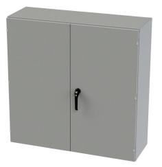
Saginaw enclosure, NEMA 3R/12/13, 48 x 48 x 16in (HxWxD), wall mount, carbon steel, ANSI 61 gray, powder coat finish, double-door, 3-point keylocking/padlocking combo handle.
