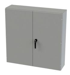
Saginaw enclosure, NEMA 3R/12/13, 48 x 48 x 12in (HxWxD), wall mount, carbon steel, ANSI 61 gray, powder coat finish, doubledoor, 3-point keylocking/padlocking combo handle.
