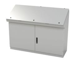
Saginaw desk console, NEMA 3R/12/13, 46 x 60 x 19in (HxWxD), freestanding, carbon steel, ANSI 61 gray, powder coat finish, double-door, 3-point keylocking flush swing handle.
