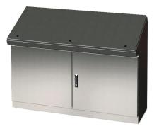
Saginaw desk console, NEMA 3R/12/13, 46 x 60 x 19in (HxWxD), freestanding, 304 stainless steel, #4 brush finish, double-door, 3-point keylocking flush swing handle.
