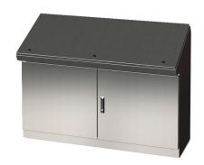
Saginaw desk console, NEMA 3R/12/13, 46 x 60 x 19in (HxWxD), freestanding, 316L stainless steel, #4 brush finish, double-door, 3-point keylocking flush swing handle.
