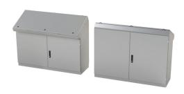
Saginaw desk console, NEMA 3R/12/13, 46 x 60 x 19in (HxWxD), freestanding, dual access, carbon steel, ANSI 61 gray, powder coat finish, double-door, 3-point keylocking flush swing handle.
