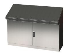
Saginaw desk console, NEMA 3R/12/13, 46 x 49 x 19in (HxWxD), freestanding, 304 stainless steel, #4 brush finish, double-door, 3-point keylocking flush swing handle.
