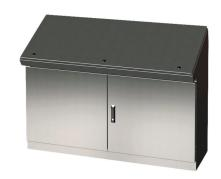
Saginaw desk console, NEMA 3R/12/13, 46 x 49 x 19in (HxWxD), freestanding, 316L stainless steel, #4 brush finish, double-door, 3-point keylocking flush swing handle.
