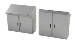
Saginaw desk console, NEMA 3R/4/12/13, 46 x 49 x 19in (HxWxD), freestanding, dual access, carbon steel, ANSI 61 gray, powder coat finish, 2-door, 3-point keylocking flush swing handle.
