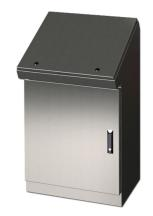
Saginaw desk console, NEMA 3R/12/13, 46 x 37 x 19in (HxWxD), freestanding, dual access, 316L stainless steel, #4 brush finish, single-door, 3-point keylocking flush swing handle.
